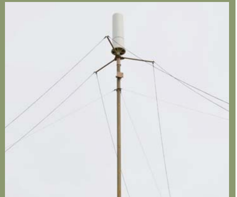
ANTI-TWIST KIT The optional anti-twist kit which is fitted to the mast head, greatly reduces torsional movement using additional guys and the special mast head attachment.
