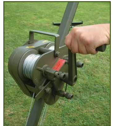
Guy winch unit (shown leg mounted but can also be ground mounted). This allows control of three guys by one person simultaneously or individually.
