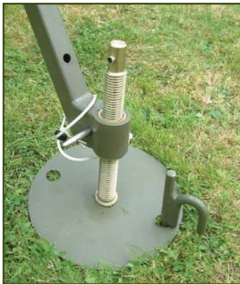
Large foot assembly for levelling the mast on sloping ground. The foot has holes for ground spikes.
