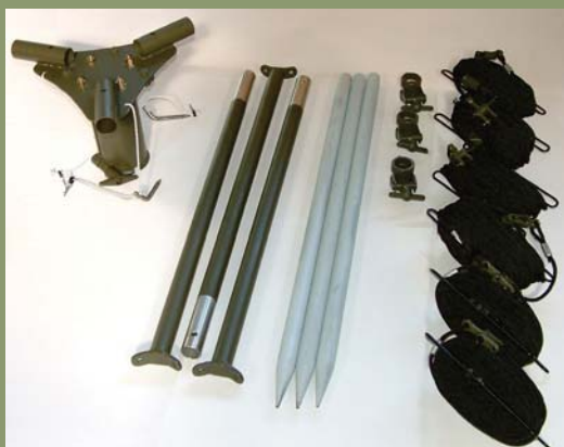
Cat. No. 44533 ANTI-TWIST KIT The optional anti-twist kit which is fitted to the mast head, greatly reduces torsional movement using additional guys and the special mast head attachment.
