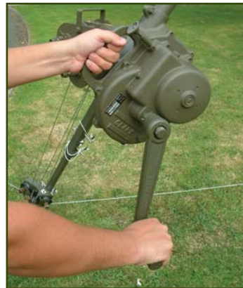
Mast hoist for raising mast sections, geared for ease of operation and only reversed by push button brake with automatic centrifugal descent control brake.
