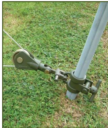
Tubular picket with guy pulley attached. Tubular pickets can be driven into the ground and the guy wire is attached at the best height regardless of ground conditions.
